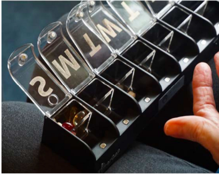
FIGURE 1. MedTracker electronic, wireless pillbox designed to track medication behavior metrics.
