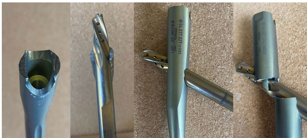
Fig. 6 Pictured from left to right: (1) Looking down at the lateral aspect of the lower half of a sectioned TFNa implant thru the proximal screw aperture. (2) The diameter of this sectioned proximal screw aperture is completely filled with insertion of the helical blade. (3) When the set screw is prematurely deployed, it acts as a mechanical block to the advancing helical blade. The blade is unable to advance any further than pictured without fracture of the locking prong. (4) Sectioned TFNa implant that has been displaced to show the direct contact of the helical blade against the locking prong when it has been deployed prior to blade/screw insertion
