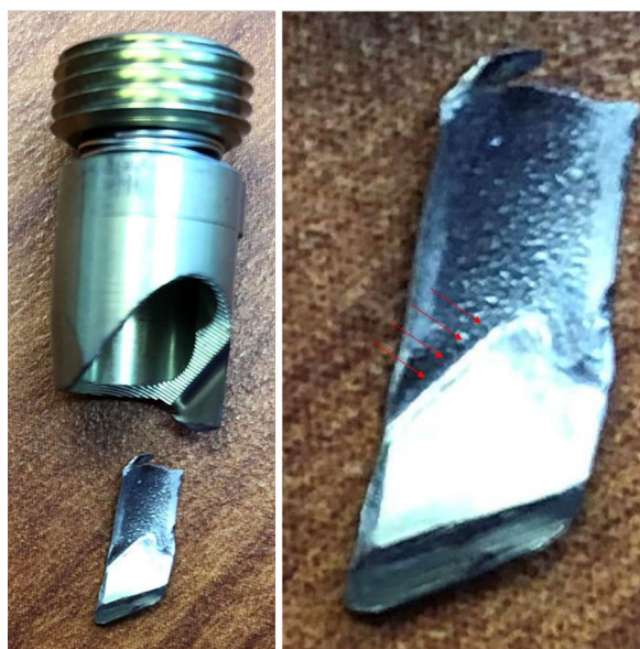
Fig. 3 A fractured set screw for the TFNa was discovered after removal and disassembly of the implant. Arrows point to engaging defect of the long prong with corresponding lesions on the helical blade consistent with fracture of the prong by the edge of the blade
