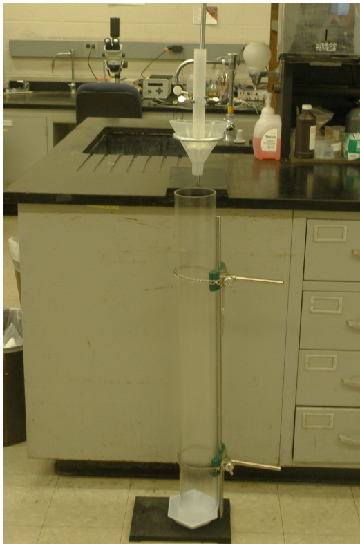
Figure 3. Flight assessment apparatus. Vials of flies are dropped through the cylindrical tube at the top of the apparatus. A ring stand holds this tube in place with a funnel. When the vial hits the bottom of the cylindrical tube flies will be ejected out of the funnel and into the acrylic tube that holds the polycarbonate sheet lined with Tangle-Trap. Flies will land along the tube and stick to their landing spot due to the Tangle-Trap.
