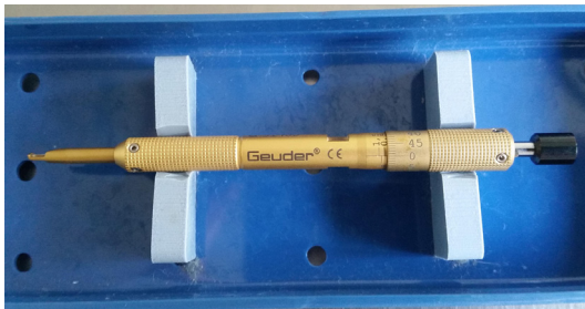
Figure 6. Diamond keratotomy knife showing Vernier adjustment to change the protrusion of the blade beyond the guard and thus determine the depth of cut
