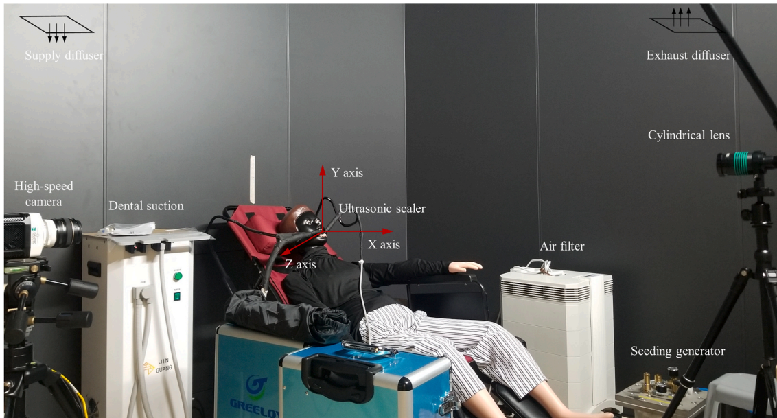
Fig. 1. The real-life photo of the experimental setup.
