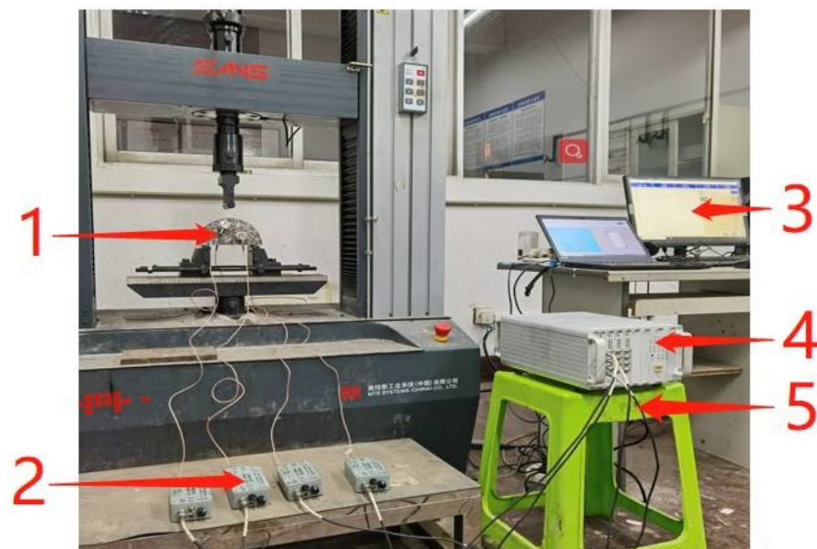
Figure 5. AE test system: 1: G8 sensors; 2: Preamplifier; 3: Computer; 4: High-speed digital AE detector; 5: Cable.
