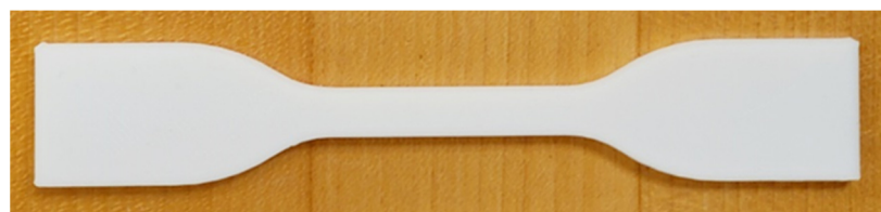
Figure 4. FDM PLA sample with a 100% infill density using Ultimaker S3.
