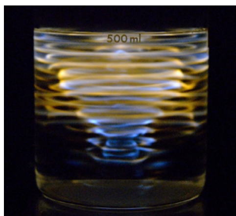
Figure 1. Photographic image of MBSL from Ar-saturated SDS solution at an acoustic power of 4 W [3]. Ultrasound at a frequency of 148 kHz was irradiated from the bottom of the beaker. Copyright 2015, with the permission from Elsevier.
