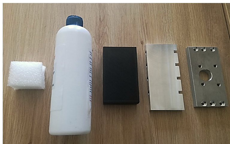
Figure 8. The five objects employed during the experiments. From left to right: styrofoam piece; soft cylinder; rigid plastic piece; metal piece; holed metal piece.
