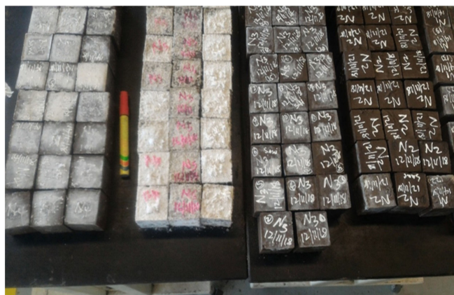
Figure 7. Extent of efflorescence formation of OPAAP.
