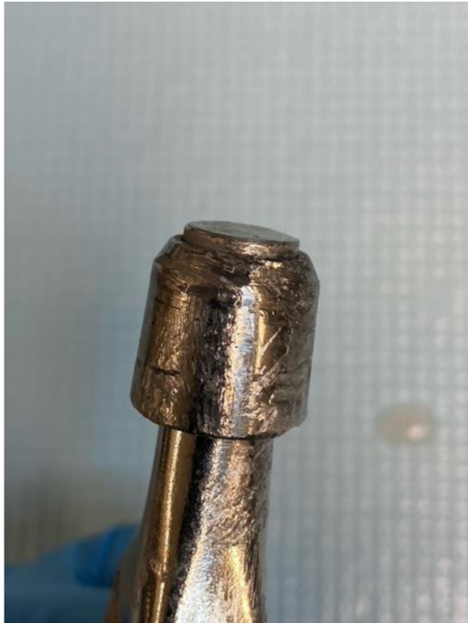
Figure 4. Clinical photograph of trunnion and sleeve after explant.
