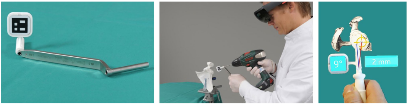
Fig. 4 AR navigated drilling of the guidewire. The HoloLens shows the planned and the current trajectory
