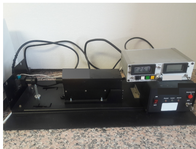
Figure 7. Custom-made NIR laser system composed of an 808 nm 10 watt F-mount laser diode.
