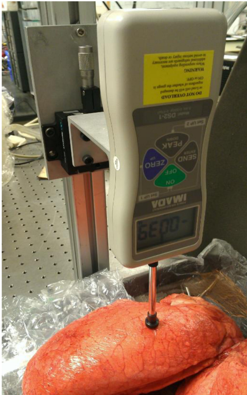
Fig. 7. Mechanical indentation test setup.
