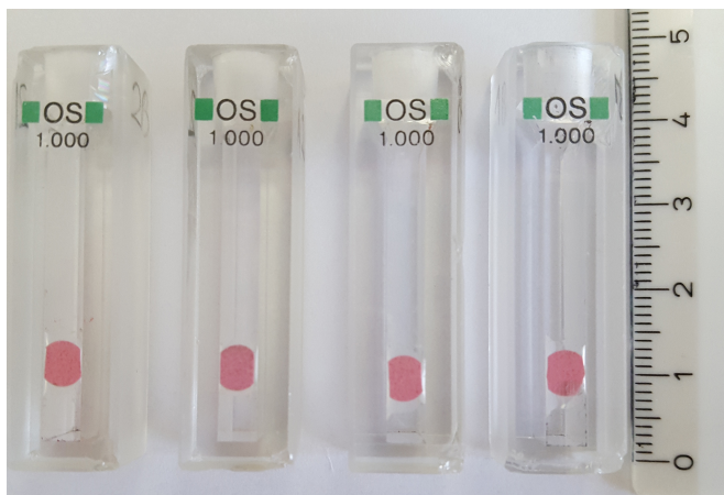
Figure 1. Oxygen monitoring cuvettes. The total volume per cuvette is 1.4 ml. A PreSens oxygen sensor spot (red) was cut and glued in place as described above.
