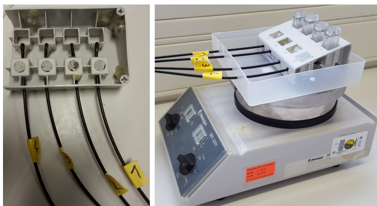
Figure 2. Images of the finished cuvette holder used to align the sensor spots glued into the cuvettes with the light conducting cable. The apparatus is placed on a magnetic stirring device to mix the reaction.
