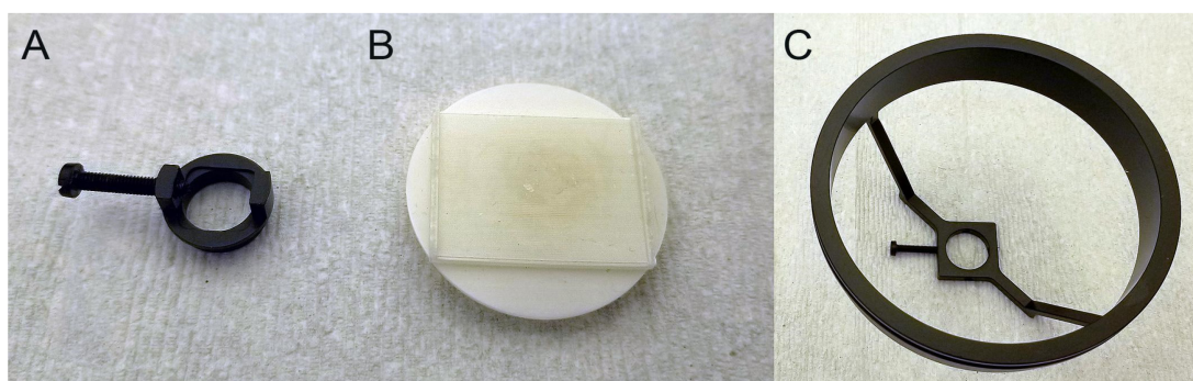
Figure 5. Sample mounting for light sheet microscopy. Sample holder for smaller agarose-embedded samples, where the sample is fixed with a screw (A). Sample holder for large agarose-embedded samples, where the sample is fixed with glue (B). The sample holder is then attached to the sample mount and fixed with a screw for submerging in DBE (C).
