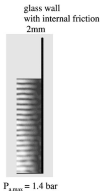
Fig. 11. The calculated spatial distribution of the acoustic amplitude for glass wall with internal friction (2 mm in thickness) [53]. The attenuation coefficient is 5 \text{ m}^{-1} . Reprinted from Ultrason. Sonochem., vol. 14, K. Yasui, T. Kozuka, T. Tuziuti, A. Towata, Y. Iida, J. King, and P. Macey, FEM calculation of an acoustic field in a sonochemical reactor, pp. 605–614, Copyright (2007), with permission from Elsevier.
