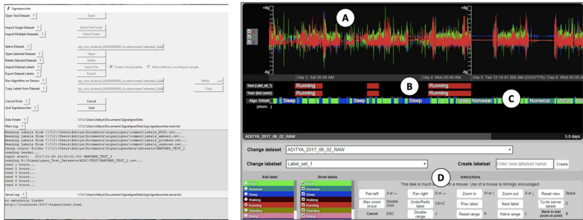
Fig. 3. (Left) Signalaligner launcher interface to import raw data and existing labels. (Right) The Signalaligner browser client displays (A) a five-day snippet from seven-days of tri-axial accelerometer data collected at 80Hz, (B) user-added activity annotations, (C) annotations from an activity recognition algorithm, and (D) data-viewing controls.
