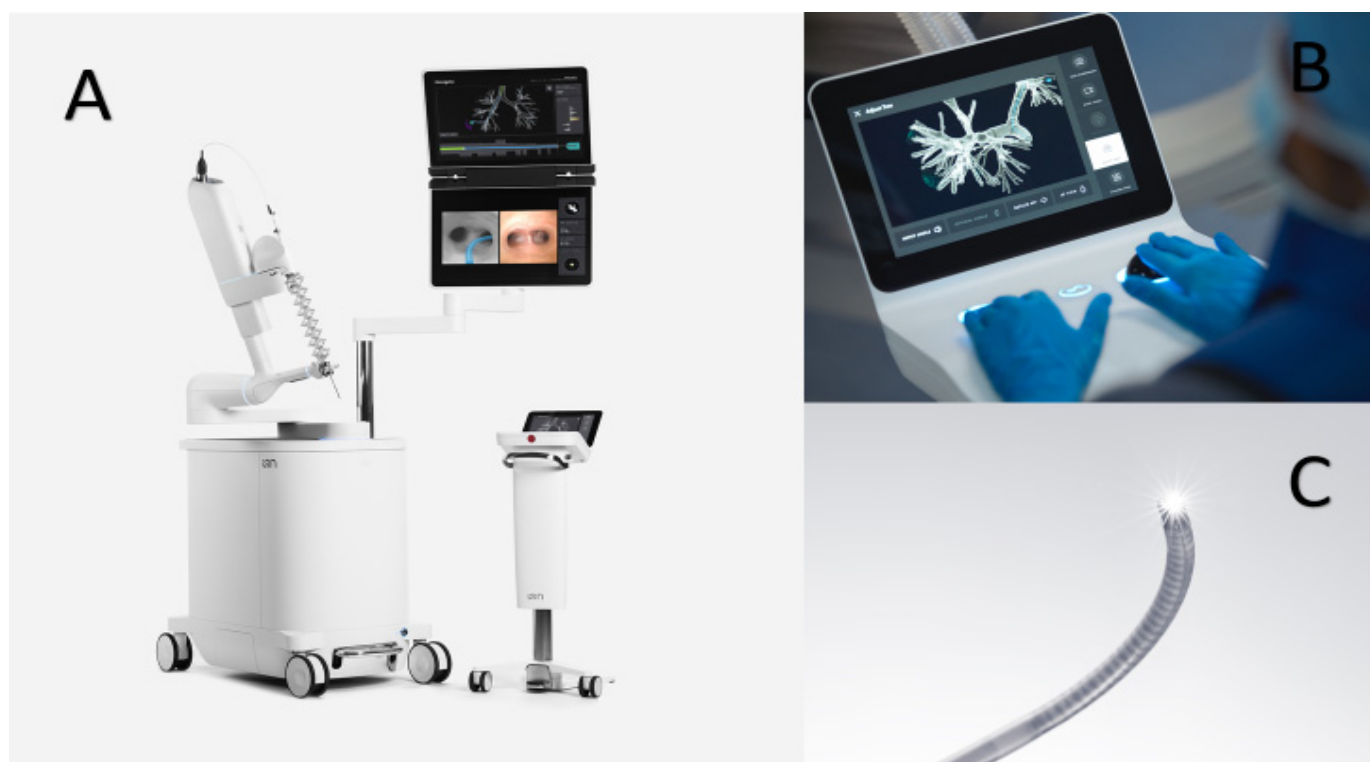
Figure 2. The Ion™ Robotic System (Intuitive Surgical). Images © (2021) Intuitive Surgical, Inc. The system consists of (A) the main system cart with articulating catheter-inner vision probe bronchoscope assembly and attached monitor plus the controller console, (B) the trackball and scroll-wheel controller, and (C) the fully articulating catheter with the removable vision probe.
