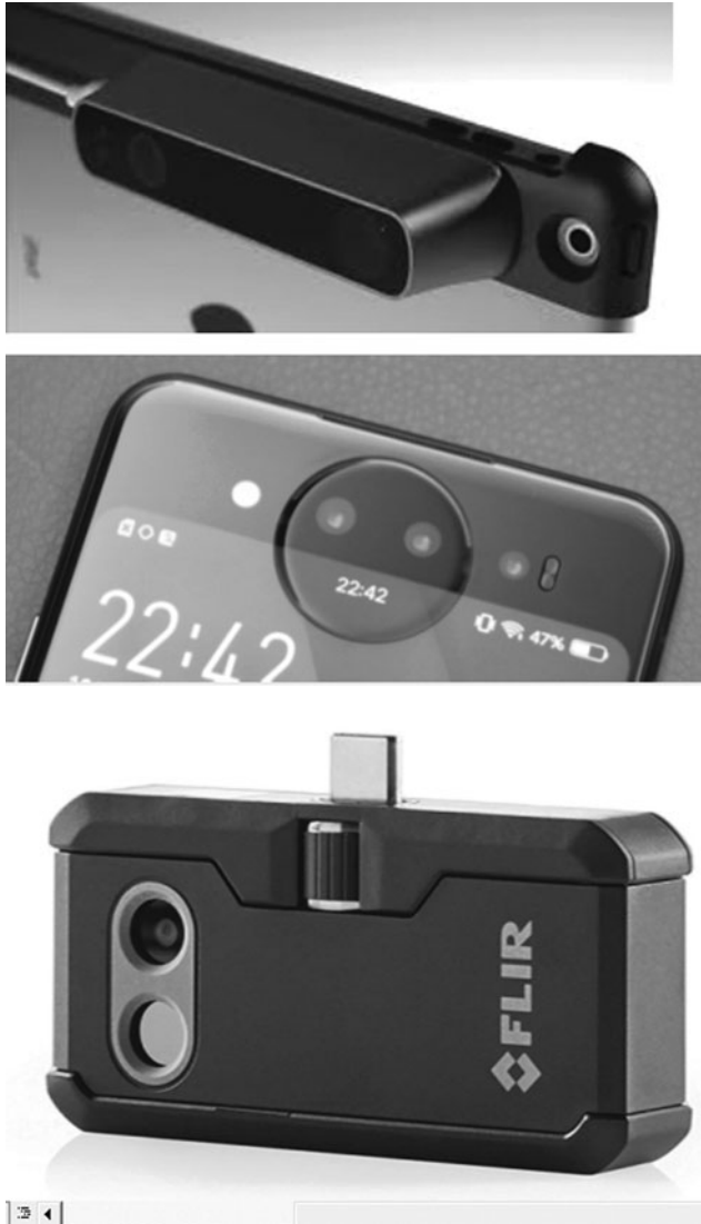
Figure 11. Structure sensor by occipital mounted on a tablet ( top ) Vivo's Nex Dual Screen TOF 3D sensor for smartphone ( center ) Flir One PRO LT thermal camera for iPhone and iPad ( bottom ). TOF, technique is time of flight.
