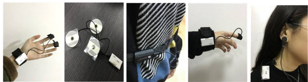
Figure 2. Biometric wearable sensing devices for measuring EDA, EMG, RESP, SKT, PPG.
