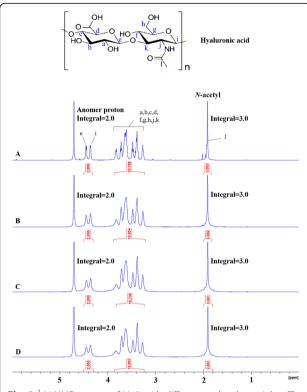
Fig. 2 <sup>1</sup> H NMR spectra of HyA with different molecular weights. The <sup>1</sup> H-NMR spectra was recorded using a Bruker Ascend<sup>™</sup> 600-MHz spectrometer, where **A** LMW-10: low molecular weight of HyA (10 kDa), **B** MMW-100: medium molecular weight of HyA (100 kDa), **C** MMW-500: medium molecular weight of HyA (500 kDa), **D** HMW-1,500: high molecular weight of HyA (1,500 kDa)
