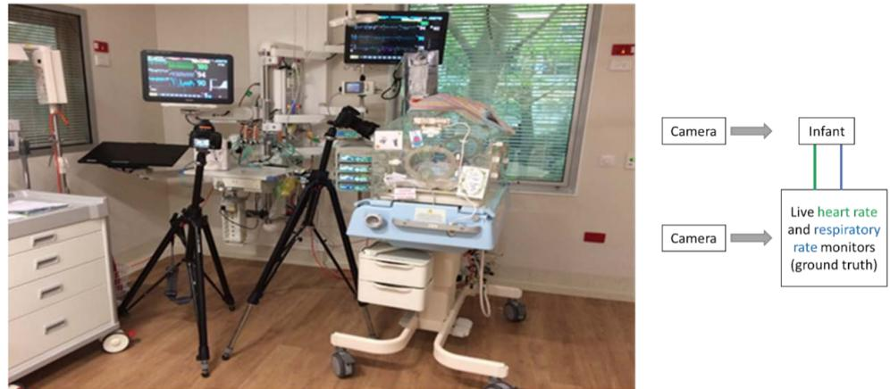
**Figure 1.** The experimental setup where the data recording was performed. A schematic of the setup is shown to the right of the image. A camera was mounted on a tripod closer to the infant to record the infant body’s heart rate and respiratory rate. Another camera was mounted on a tripod to capture vital signs’ ground truth (shown on the monitor). A schematic diagram on the left of the figure shows an overview of the setting.
