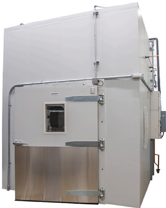
Fig. 1. Walk-in environmental chamber (Labworks Internationals Inc.) used to create simulated environmental conditions by controlling temperature and humidity.
