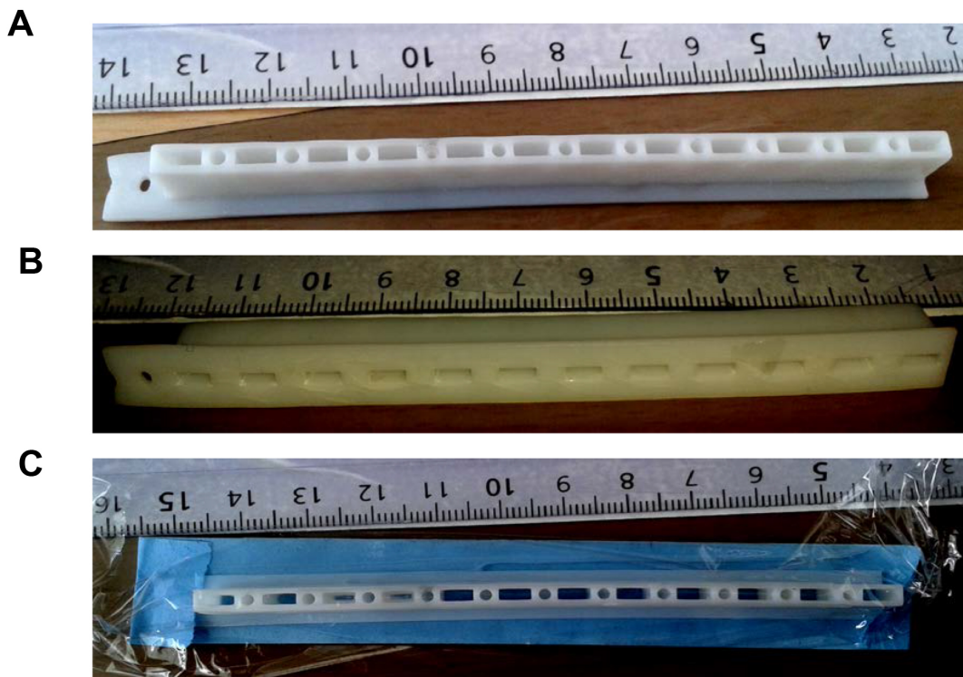
Figure 2. Pictures of a plug mold. A and B. Top and bottom views; C. Plug mold sealed with a tape and covered with a saran plastic film.
