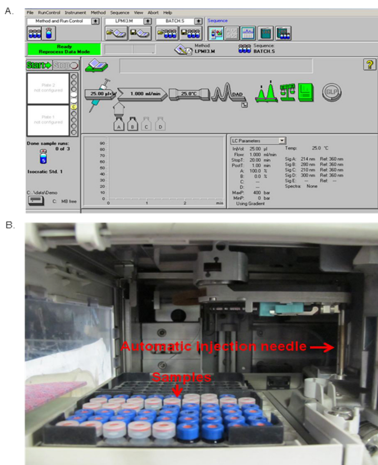
Figure 3. HPLC program and instrument. A. HPLC program in ChemStation Software; Rev. A.10.02 [1757]. B. A part of HPLC machine indicating samples orientation and automatic injection needle.
