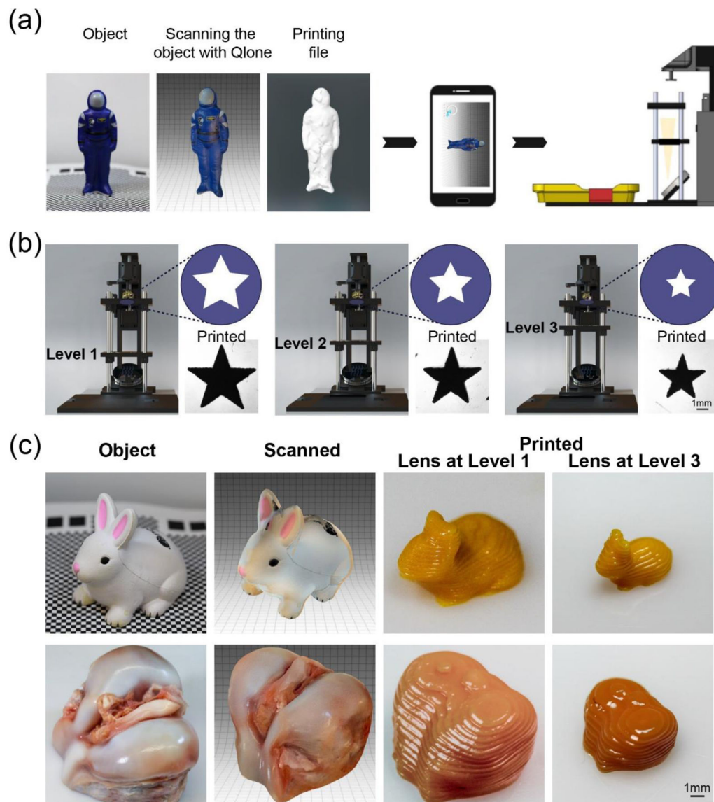
Figure 5. Integration of the smartphone 3D scanning App. (a) Scheme showing printing with the model obtained from the 3D scanning App. (b) Various magnifications achieved from 1.5 to 1.0 times through adjusting the level of focusing lens from Level 1 to Level 3. Images in right-bottom corners present printed constructs exposed to the same projecting pattern that was passed through different focusing lenses. (c) 3D-printed bunny toys and femoral condyle constructs with Level 1- to Level 3-magnifications.
