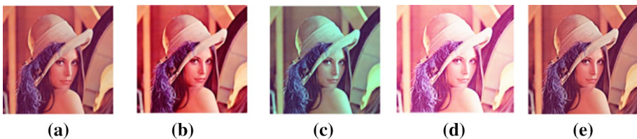
Fig. 9 Output images from applying different filters, a original image, b histogram equalization, c white balancing, d enhancing brightness, and e sharpening
