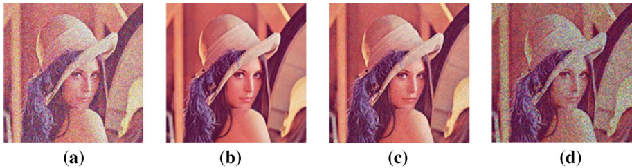
Fig. 11 An example of different noises a Gaussian noise, b Poisson noise, c salt & pepper noise, and d speckle noise
