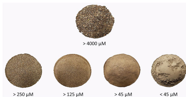
Figure 1. Brown macroalgae S.cristaefolium and their corresponding thallus grounded to different particle sizes.
