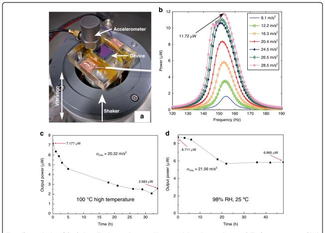
**Fig. 5 Characterization of the device. a** The device is characterized by using a shaker with an accelerometer; **b** The frequency response of RMS powers vs. frequencies at different accelerations; The maximum RMS output power of the device after being placed **c** on 100 °C hotplate and **d** in 98% RH, 25 °C humidity cabinet for different time
