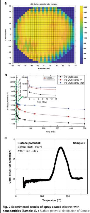
5 after corona charging, **b** surface potential decay over 500 days, and c open-circuit TSD current spectra of Sample 5
