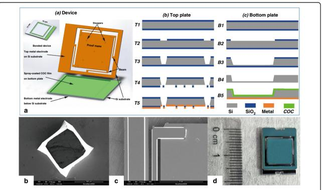
**Fig. 4 Fabrication process of the energy harvester device and its photos. a** Schematic and fabrication process of the electrostatic energy harvester device, which is composed of a top plate and bottom plate with MEMS technology, SEM images of the **b** stopper and **c** beam on the energy harvester device with corner compensation, and **d** electrostatic energy harvester after low-temperature bonding. The size of this whole device is  $13 \times 18 \text{ mm}^2$
