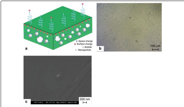
**Fig. 1 The proposed spray-coating method for electret material with nanoparticles. a** Schematic of the electret material deposited by spray coating and small bubbles and PS nanoparticles are introduced by spray coating, which could be helpful for trapping more space charges; **b** photograph of a spray-coated electret with many bubbles; **c** SEM image of a nanoparticle on an electret layer; Table 1: Samples prepared by spin and spray-coating methods
