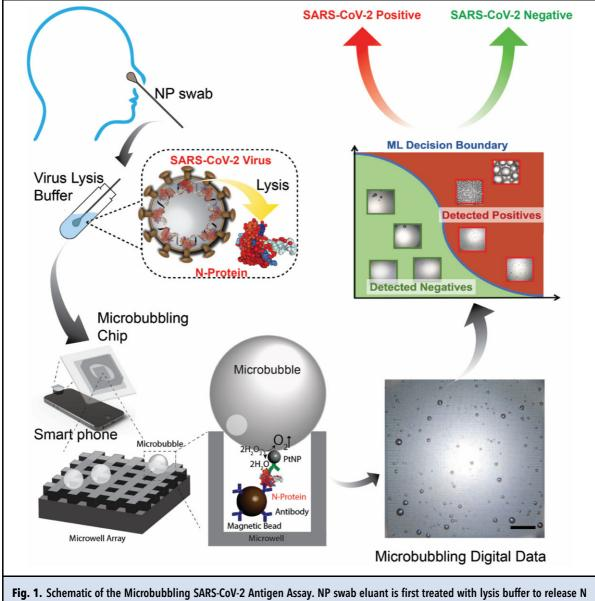
Fig. 1. Schematic of the Microbubbling SARS-CoV-2 Antigen Assay. NP swab eluant is first treated with lysis buffer to release N proteins from SARS-CoV-2 viruses. N protein is then detected by the smartphone-based microbubbling digital assay. The microbubble images are quantified and classified as positive or negative by computer vision and ML algorithms. Scale bar, 500 μm.
