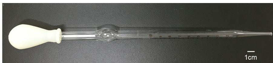
Figure 6. Komagome pipette (10 ml) with silicone rubber bulb
