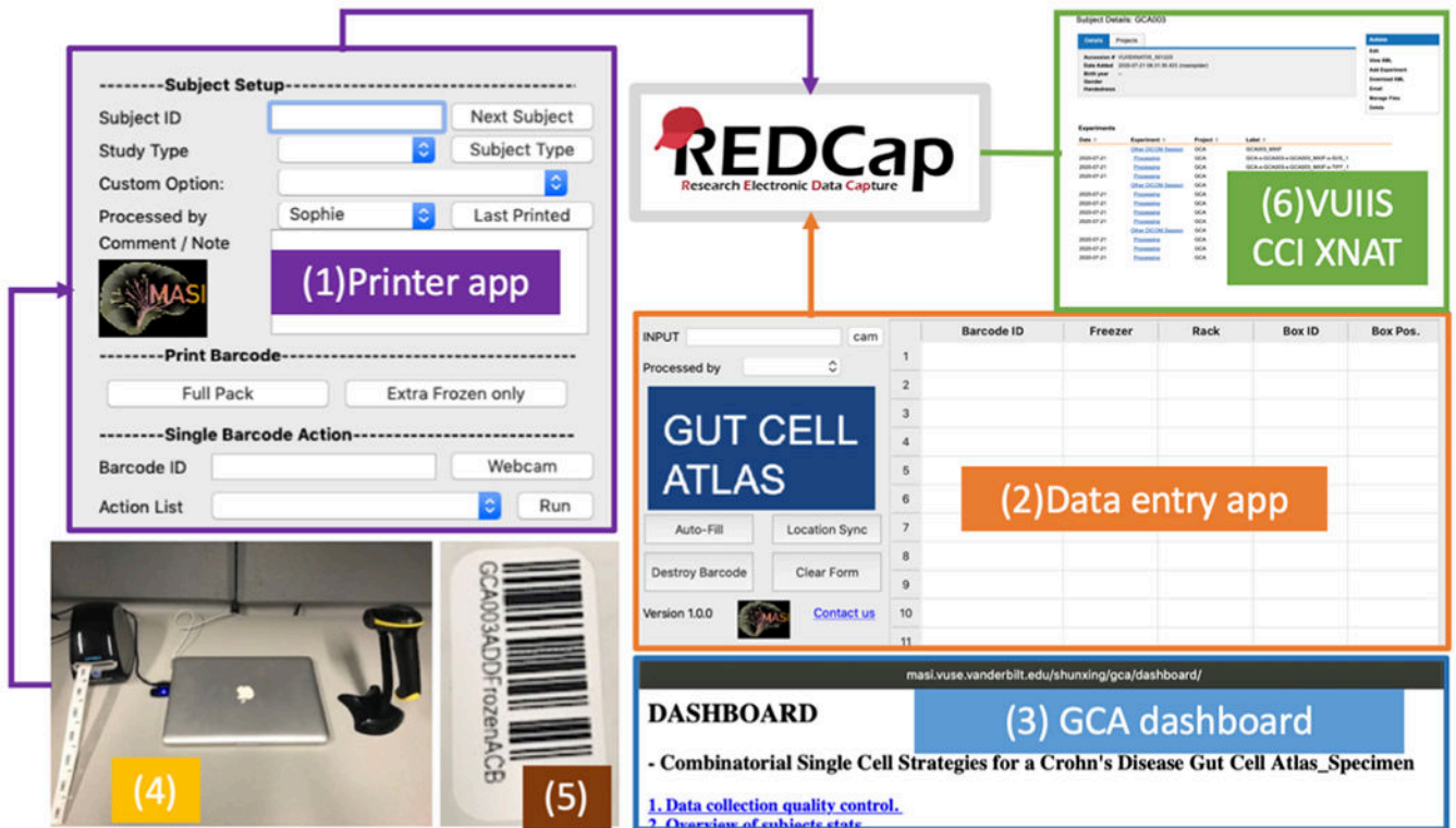
Figure 2. The data entry workflow of the GCA data collection. (1) According to patient types (i.e., healthy control vs Crohn’s disease), the printer app generates the barcodes). The barcodes are recorded to REDCap after printing. The barcode is human-readable, and scanner scannable for any further sample operations (i.e., distribute to other labs, store to a rack & box position, destroy a barcode). (2) The Location/Data entry app is a user-friendly software to help users enter data into REDCap to reduce manual input errors. (3) The GCA online dashboard is designed to show sample stats that users may care about, and it also allows for quality control and identification of potential inconsistencies with data entry in REDCap. (4) All apps are installed on a laptop workstation. The workstation connects to a barcode label printer and wireless barcode scanner. (5) A sample barcode for a frozen specimen. (6) The VUIIS CCI is a system based on XNAT that is used to store any large data in the GCA project.
