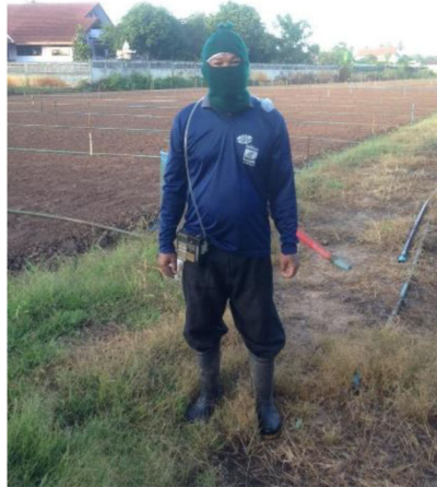
Figure 2. The breathing zone air sampling (a) and patches sampling on bare skin of farmers on 10 locations, right and left upper arm, forearms, upper legs, lower legs, forehead, and back (b).
