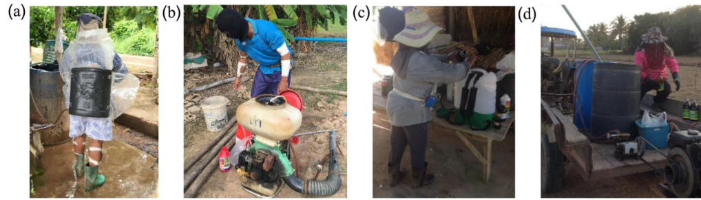
Figure 1. Type of spraying equipment: (a) manual pump backpack; (b) motorized spray backpack; (c) battery pump backpack; and (d) high pressure pump.
