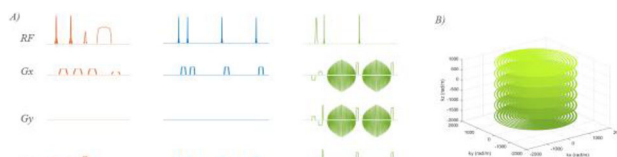
Figure 1. A) Sequence diagram of SOSP ASL acquisition, orange-blue: FAIR-QUISSII labeling module, green: SOSP readout with fat saturation. B) SOSP trajectories, the acquisition started from the bottom of the kz plane and moved upwards linearly
