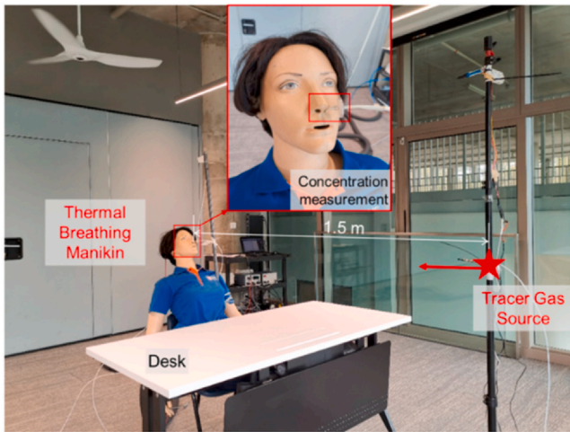
Fig. 18. A manikin position with tracer gas source and aerosol sampling probe (Li et al., 2021).
