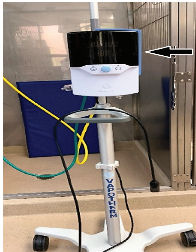
Figure 1. High-flow oxygen machine (Precision Flow Plus; Vapotherm, Exeter, New Hampshire, USA). The yellow hose is attached to medical/compressed air, the green hose is attached to the oxygen source and the black cord connects to the power source. The flow generator and humidifier are contained within the unit (black arrow).
