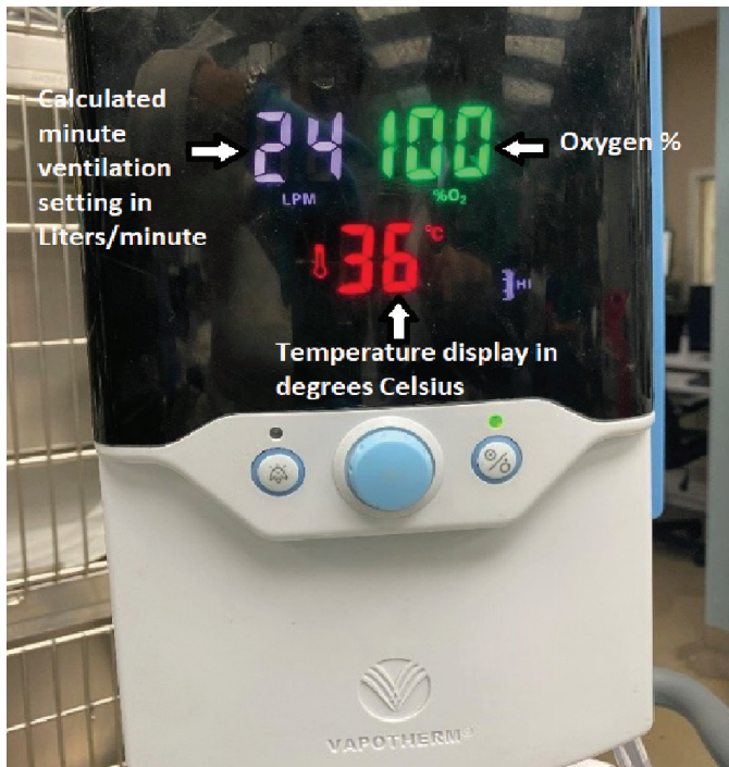
Figure 5. High-flow oxygen machine display. Photo courtesy of Dr. Mariana Pardo, MV, BVSc, DACVECC.
