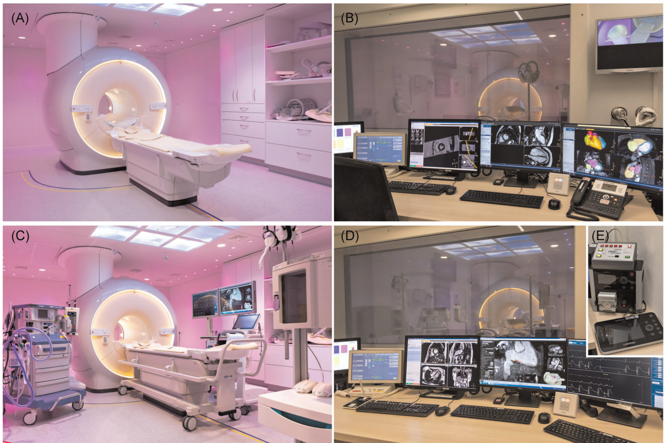
FIGURE 2 Full transformation of the pre-existing MRI environment into an interventional cardiac MRI suite. (A) pre-existing diagnostic MRI scanner room. (B) pre-existing diagnostic MRI control room. (C) transformed iCMR suite (from left to right: anesthetic equipment, contrast pump, MR scanner with transportable tabletop, two movable displays (left EP recordings, right real-time MR imaging/active catheter tracking), patient vitals monitor, wireless communication headsets, MR safe anesthetic infusion pump cabinet). (D) transformed iCMR control room (the two right monitors correspond to the displays inside the iCMR suite). (E) the non-MR compatible RF generator including cooling-pump positioned in the iCMR control room. EP, electrophysiological; iCMR, interventional cardiac MRI; MRI, magnetic resonance imaging
