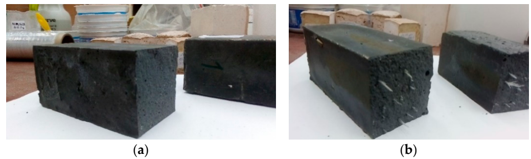
Figure 9. Breakthrough of samples based on fly ash (a) without reinforcement; (b) with 0.5% addition of glass fiber.
