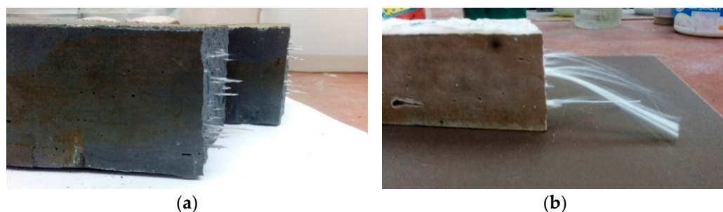
Figure 12. Changing the behavior of glass fibers placed in various geopolymer matrices: (a) fly ash-based matrix; (b) metakaolin-based matrix.
