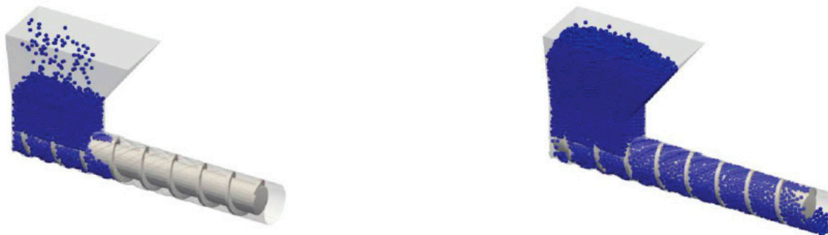
Figure 5. Overview of a DEM simulation of spherical particles—reprinted with permission from [22], with the permission of AIP Publishing.
