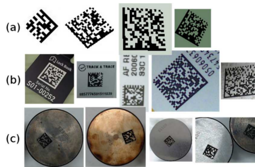
Figure 19. Testing samples: (a) synthetic; (b) Internet; (c) industrial.
