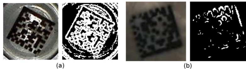
Figure 20. Edge detection problems: (a) Merged edges; (b) Missing edges.
