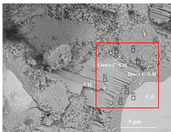
Figure 2. The BSE images of partially hydrated C 3 S particle after 28 d.
