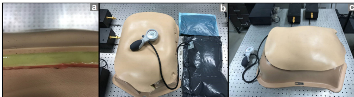
Figure 1. Abdominal wall phantom used in the in vitro study. (a) The multi-layer structure of the artificial abdominal wall, representing skin, fat, muscles, fascia, and peritoneum. (b) Artificial abdominal compartment in addition to water- and air-filled balloon to simulate different case scenarios in intra-abdominal hypertension. IAV was increased via the air-filled balloon, which subsequently resulted in intra-abdominal pressure (IAP) elevation. (c) The final assembly of the abdominal wall phantom studied by transient radar method (TRM).
