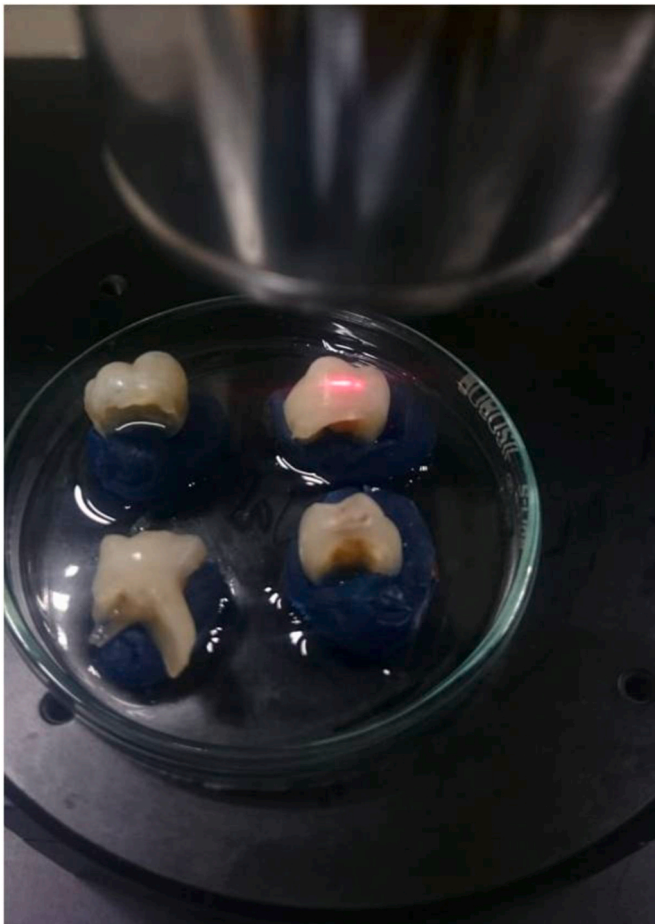
Fig. 1. Scanning of samples with SS-OCT.
