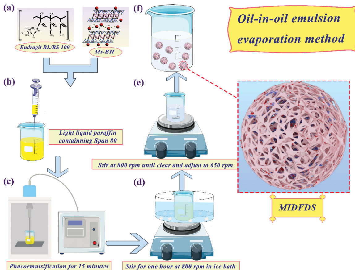
Figure 1. Schematic diagram of the preparation process of MIDFDS using the oil-in-oil emulsion evaporation method.
