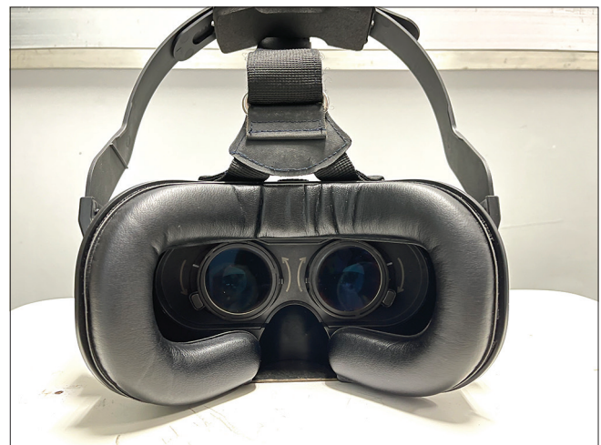
Figure 3: Image of advanced vision analyzer (AVA, Elisar) showing compact rimming and a snug fit enclosed chamber over the periorbital region, to provide dark room effect and also providing a barrier to aerosol internalization
