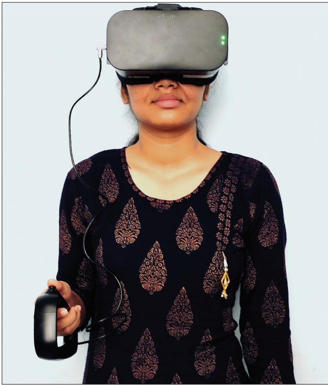
Figure 4: Image shows the complete externalization of the nose outside the perimetry chamber, hence preventing contamination of the enclosed space
