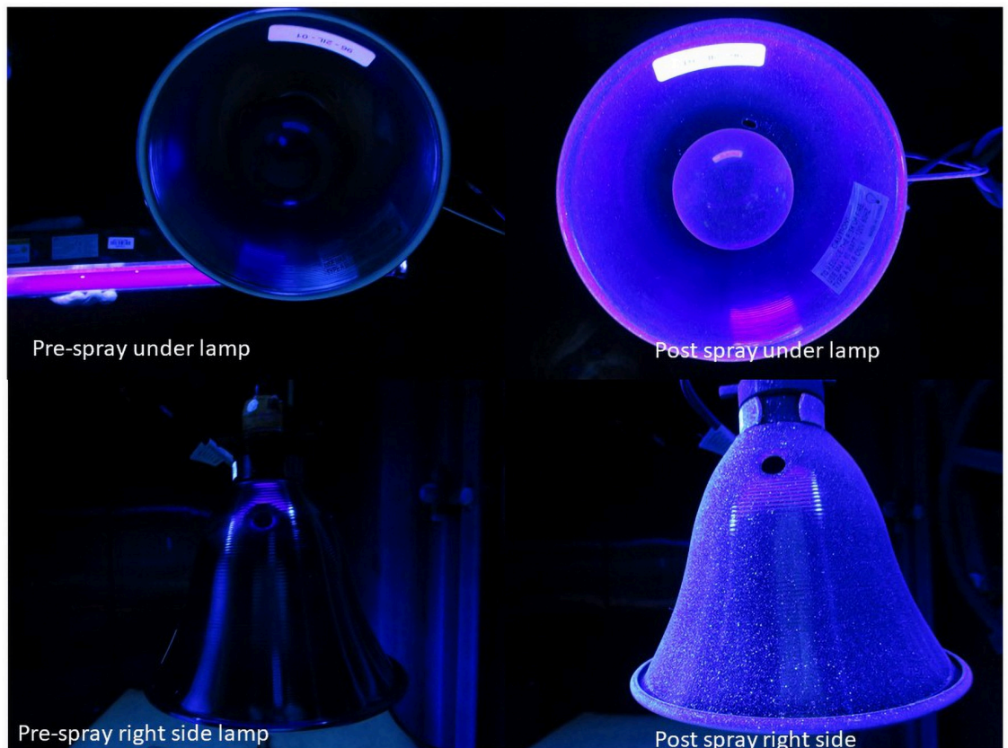
Fig 5. Example photographs of a clip-on lamp, before and after spraying fluorescent dye solution.
