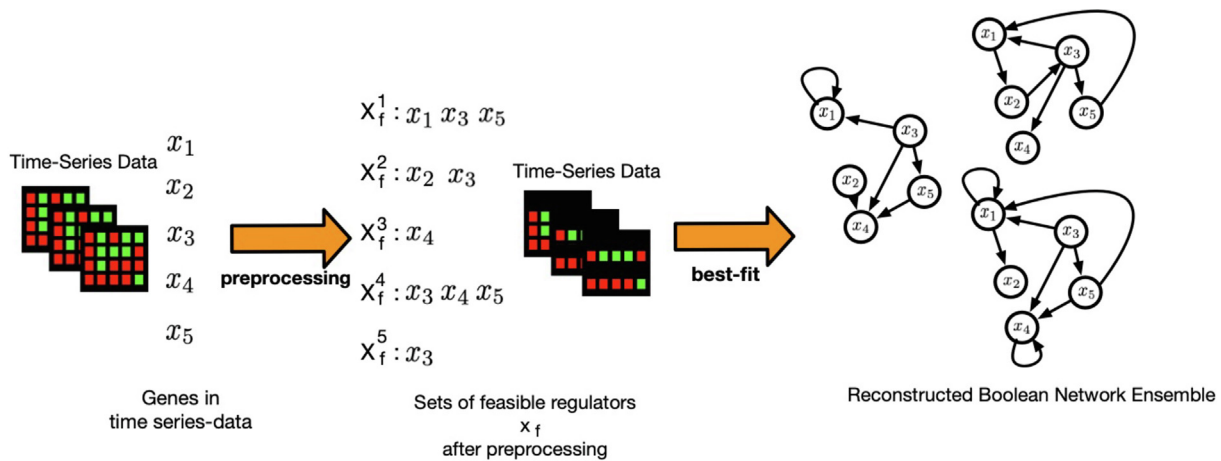
Fig. 2. Overview of the new Boolean network reconstruction pipeline. The Boolean networks reconstruction pipeline combines a correlation-based approach to predict regulatory inputs by Maucher et al. [30] and the Best-Fit Extension algorithm by Lähdesmäki et al. [31]. The algorithm by Maucher et al. is used as preprocessing step to reduce the number of inputs that will be tested for the succeeding est-ixtension algorithm. This combination decreases the reconstruction time without losing meaningful results.
