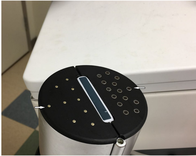
Fig. 2. US-guided DOT probe. The foot-print of the combined DOT probe is approximately 10 cm. Four source laser diodes of 730 nm, 785 nm, 808 nm and 830 nm optical wavelengths were sequentially switched to nine source positions (pointed by an arrow) on the probe, while the reflected light was coupled by the 14 light guides (pointed by an arrow) to 14 parallel detectors
