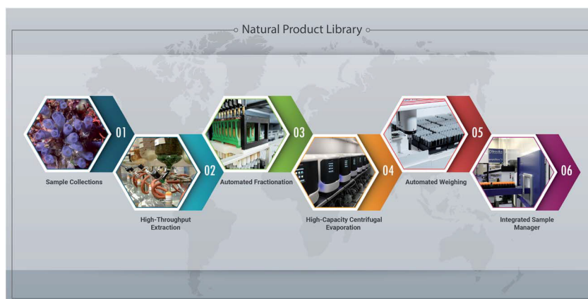
Fig. 2. Overview of automated and high-throughput processes developed at the NCI National Program for Natural Products Discovery (NPNPD) to facilitate the production of a natural product-based screening library. (1) Since 1986, more than 80 000 samples have been acquired through collection agreements based on the NCI letter of collection with each participating source country or their representatives, which stipulates equitable benefit sharing from commercial products derived from discoveries made through these collections. (2) Extracts in the NCI NPR are prepared in a high-throughput manner using both an aqueous and organic solvent extraction process, resulting in two sequential extracts per collected specimen/sample. 27 At present, the US National Cancer Institute's (NCI) natural product repository contains over 230 000 unique extracts derived from plant, marine and microbial organisms. (3) Extracts ( n = 88 ) are prefractionated on a customized Positive Pressure Solid Phase Extraction workstation (PPSPE) with two robotic arms working in parallel to produce seven fractions per extract (3.5 h; n = 616 fractions). (4) Fractions are dried using high-capacity centrifugal evaporation systems (18 h; n = 2304 ), and the final mass of each fraction is determined on an automated weighing station (5). (6) An automated sample management system with the capacity to store 1.1 million 2D-barcoded tubes (10 ml) is integrated with robotic systems designed to generate 384-well microtiter plates for HTS and 96-well plates for secondary HPLC-based fractionation of active primary fractions.
